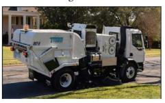
The **Tymco Model DST-6** pick-up head has a width of 87 inches and is equipped with a broom in the pick-up head for applications where a broom is desired. The fast rotation of the broom loosens packed-on debris and projects it into the Regenerative Air stream for effective cleaning.
