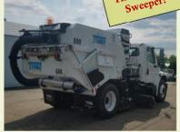
This Tymco 600BAH offers a 6-Yard capacity, Diesel JD 4045T T4 99HP Engine, Stainless Hopper & Housing, Dual Digger RH Tilt Gutter Brooms, High Output Water, Air Purge ASI, PHU Curtain Lifter, and Sweeper Deluge, along with tons of additional features!
