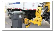
Long, slender, straight grabber geometry – gives you the ability to reach in tight places and spear cans. Can Weighing: Ability to set max threshold of 350lbs - will halt the lift automatically if cart is overweight. Joystick Functions – Can Shake, Pick Height, Pick Angle. Functions can all be adjusted and used via the 5-button joystick.
