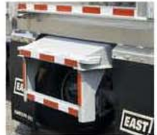
Subframe integrated with push block.
