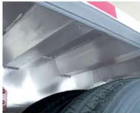
Aerodynamic V-shaped cross-members.
